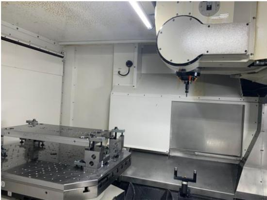
The swivel axis of the Mikron HPM 1850U also allows optimum access to the workpiece from the side. A high surface quality is achieved even during simultaneous machining. The Step-Tec Spindle offers full torque even at low speeds.
