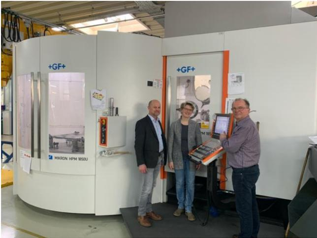
The Mikron HPM 1850U has a tool magazine with 238 positions. This means that sufficient tools and the sometimes necessary sister tools can be stored, even if the individual pallets have different requirements.
