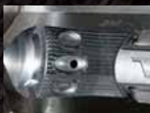
Engrave in mould for rubber industry (Automotive) material: steel
