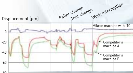
Thermal displacement of the tool origin (Z-axis) under different machine loads.
