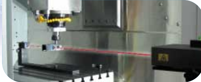
Axis positioning check in compliance with ISO 230-2
