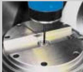
Hole in the centre Reference pallet "MacroMagnum"
