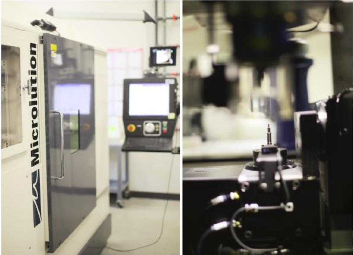
*Laser machining station with detail*
