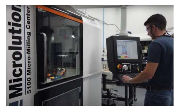
On the micro-milling side, Sunlight-Tech's Microlution 5100 Micro Milling Center gives the shop the ability to produce highly precise parts with complex geometries.
