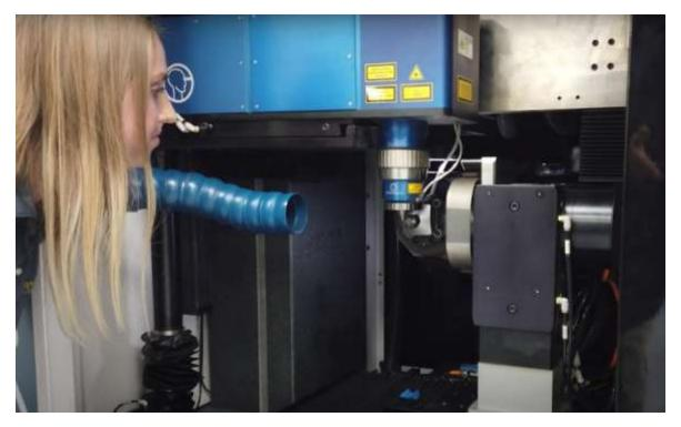
The femtosecond lasers inside the machines have ultrashort pulses in the range of one quadrillionth of a second.
