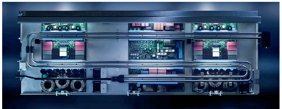
The innovative Intelligent Power Generator (IPG) from AGIE CHARMILLES, part of UNITED MACHINING enables digital and precise control of every spark and is extremely energy-efficient
