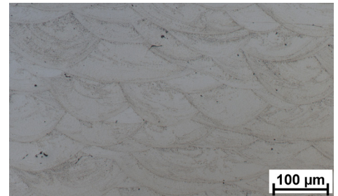
Microstructure without heat treatment (NHT)
