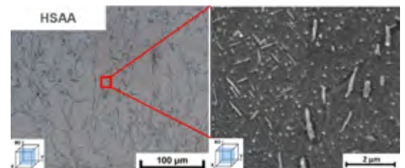
Microstructure after HSAA
