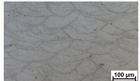
Microstructure after SR
