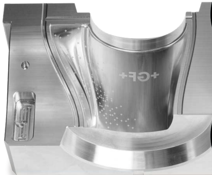
Tempering by conformal cooling channels
