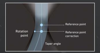
TAPER-EXPERT allows very precise machining of tapers with angles varying from 0 to 30°. It corrects in real time and during machining the position of the wire depending on the angle. The surface quality is the same as with in cylindrical machining.
