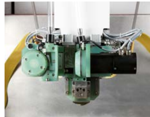
Automatic Wire Changer (AWC)
