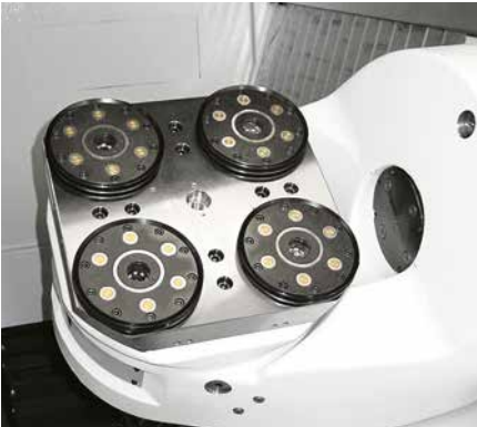
Delphin reference system vibration damping for better surface quality.
