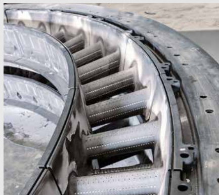
Tight seal slot reduces turbine leakage.
