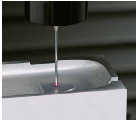
Touch probe included in the head guarantees high positioning accuracy.
