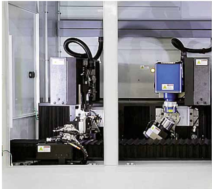
Dual five-axis stations to combine Milling and Laser machining.
