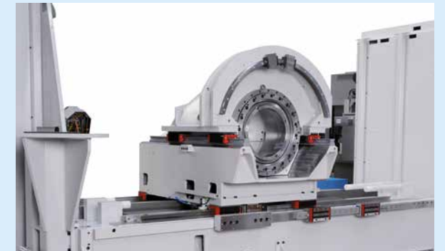
Rigid, compact layout of all axes for high jerk machining.
