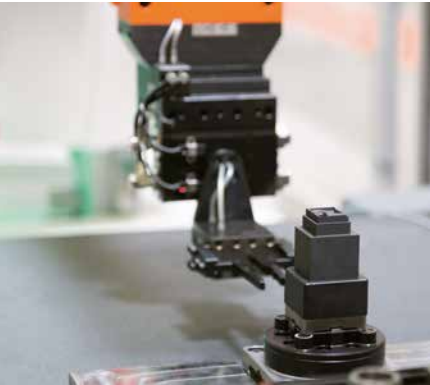
Complete range of clamping systems can easily adapted to any part or electrode.
