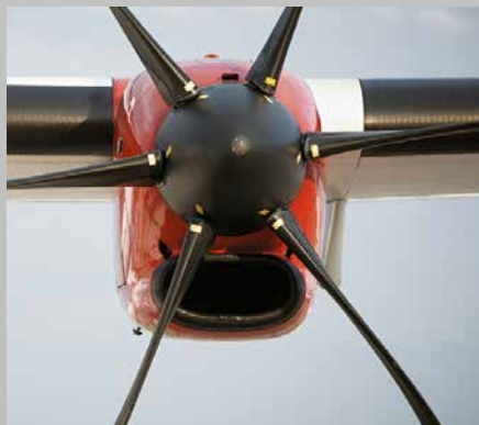
Composite blades need protective metal leading edge.
