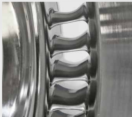
Complex 3D airfoils with small root radii.
