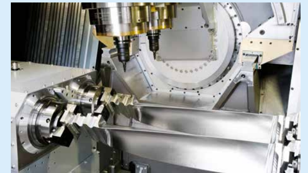
Twin Spindle machining with automatic tool length compensation.
