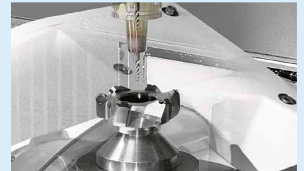
By accessing part from all directions, five-axis machining can finalize complex features initiated in Additive Manufacturing.
