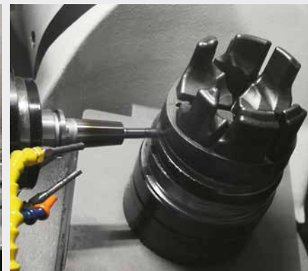
Improve surface finishes and small shapes requiring five-axis Milling.
