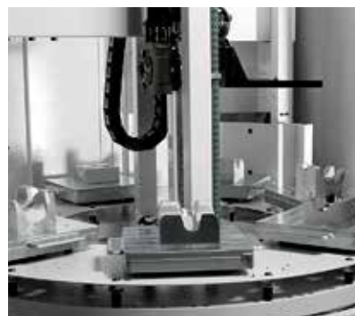
Integrated pallet magazine Automation Maximize your productivity and autonomy while producing at lowest cost.
