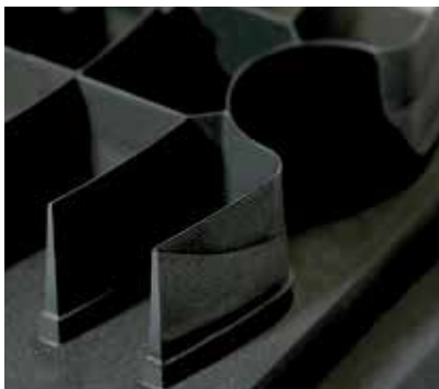
iGAP and wear partitioning technologies Deep, thin, sharp corners; uniform results on multi-cavities.
