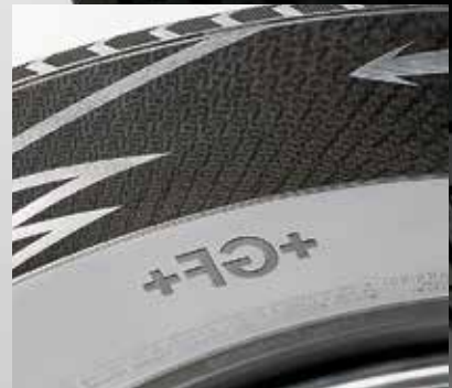
Sidewall texturing, engraving: Fully digital, unlimited design possibilities, no tooling inventory
