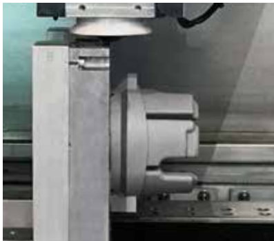
Separation from build plate is needed for 100 percent of additively manufactured parts
