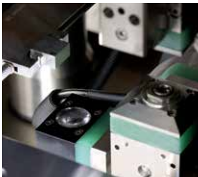
Integrated Vision Unit (IVU Advance) In-process measurements for closed-loop processes to achieve highest accuracies.
