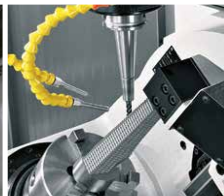
High-speed five-axis machining improves surface finishing and reduces post-processes like polishing or grinding.
