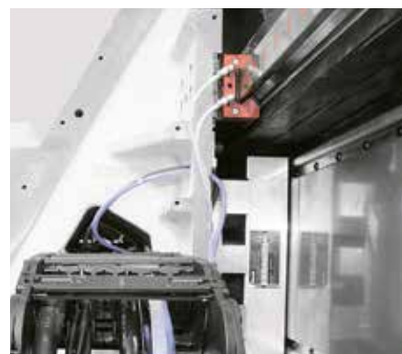
Linear precision guide reduces machining time and produces better surface finish on orthopedic implants.
