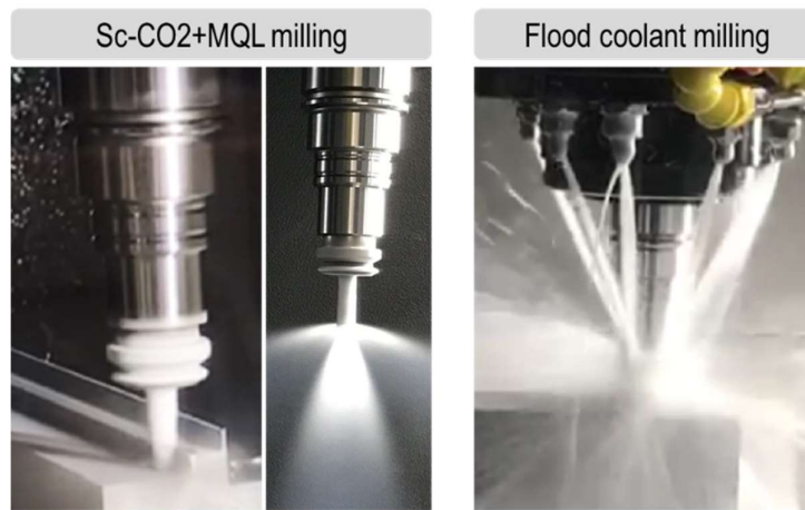
Figure 1. High-speed side milling under Sc-CO 2 +MQL (left) and flood cooling (right)
