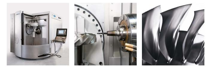
Designed for the production of airfoils with 5-axis simultaneous machining technology. Efficient roughing and dynamic finishing in 1 setup.
