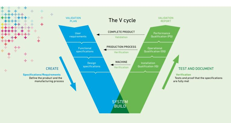
As part of the documentation needed for compliance with 21 CRF 820, or ISO 13485, this document establishes proof that critical connections to utilities, and status of the equipment, are meeting GF Machining Solutions instructions.
