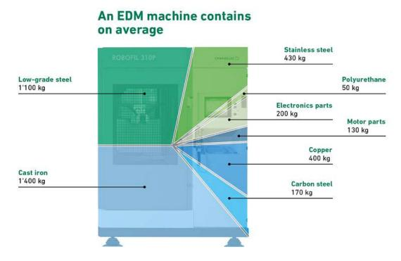
The parts and materials used for EDM machines are obtained from scarce resources.
