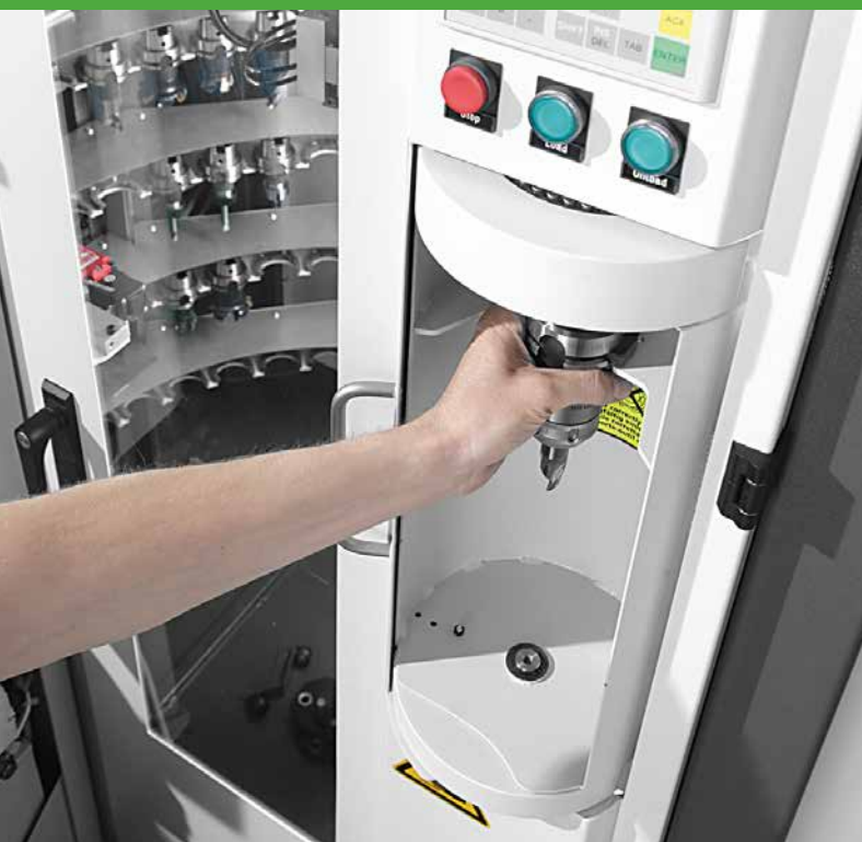
Circular magazine design with handling system
