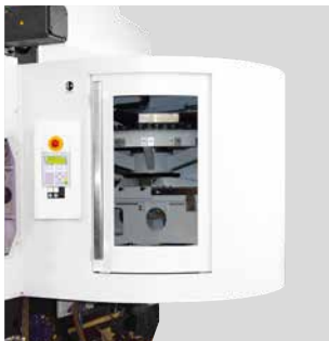
Tool magazine HSK-A/T100: 30 tools HSK-A/T63: 45 tools
