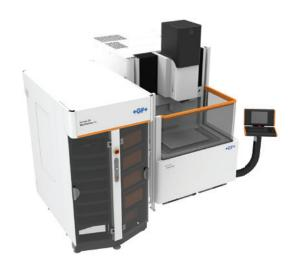
WorkPartner 1+ Entry designed for single EDM machines. 3 to 5 pallets for workpieces together with a remarkable number of electrodes. The unit includes a Load station and a Drain station to make everyday work easier, in less than  $4m^2$  floor space.
