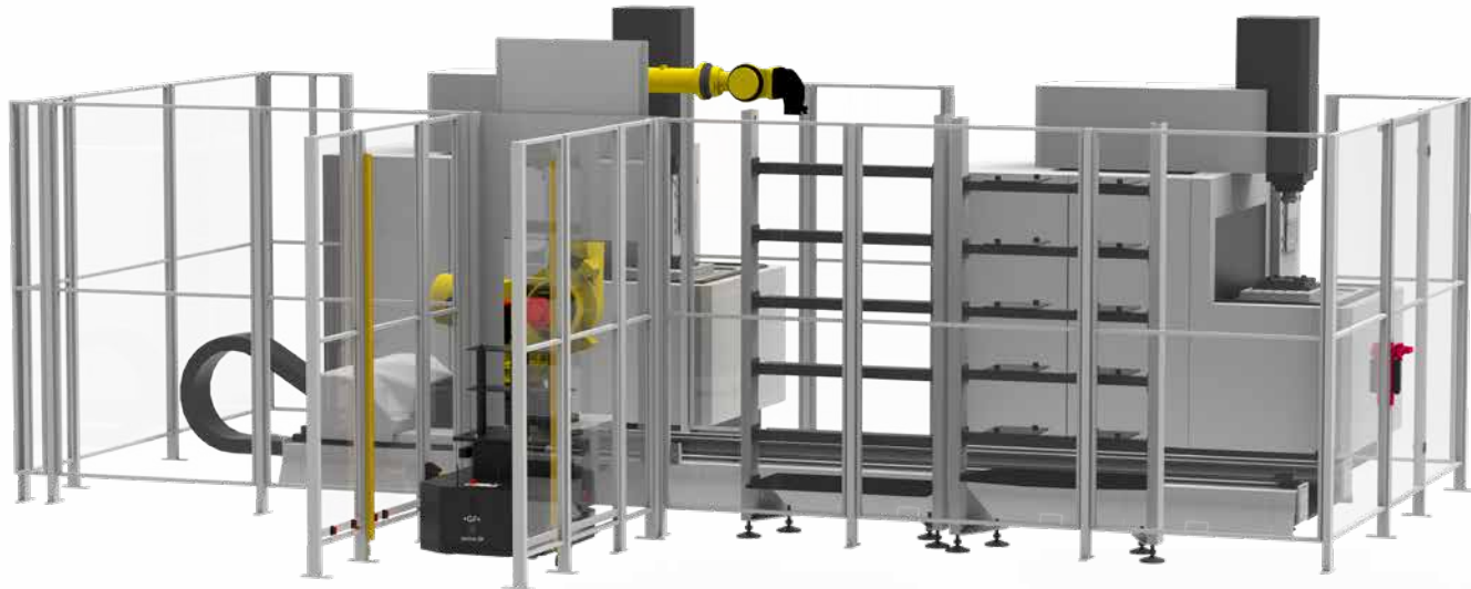
Transformer 6-axis: AMR with tray and lifter at a loading/unloading station.
