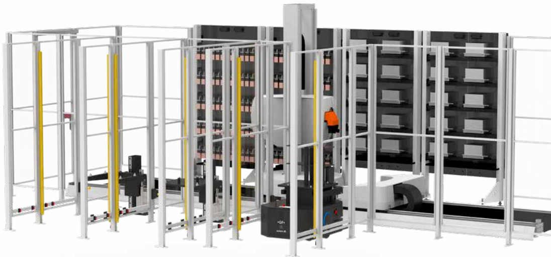
Transformer 3-axis: AMR with tray and lifter at a loading/unloading station.
