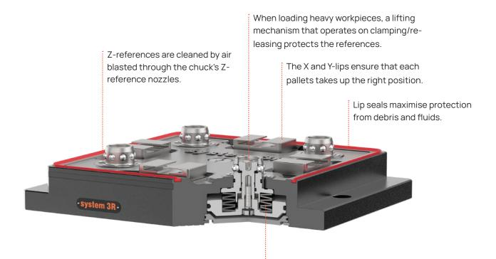
Spring-loaded when idling; special Turbo function via added air pressure.
