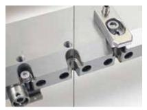
Clearance for wire between workpiece and ruler.
