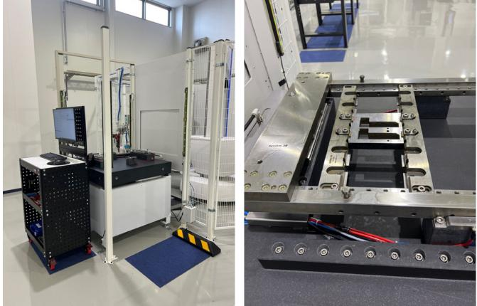
WEDM Cell with CUT P 550 Pro, stationary Transformer, Rack magazine for the WEDM Frames and CMM outside the cell also used as loading station for the large WEDM frames
